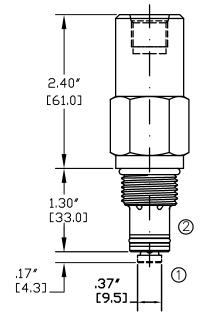
NOTE: CAVITY BOTTOM HOLE MUST ALLOW FOR POPPET EXTENSION (.500 DIA) FOR ALUMINUM OR STEEL VALVE HOUSING CONFIGURATIONS SEE PAGE 0-012.1
